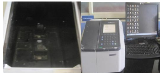
Figure.1: Shimadzu UV-Visible Spectrophotometer with quartz cuvettes and digital display.
