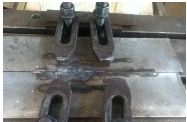
Fig.2. Material clamped on FSW machine
