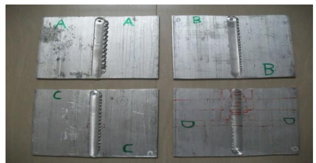
Fig.3. Friction Stir Welded specimen's
