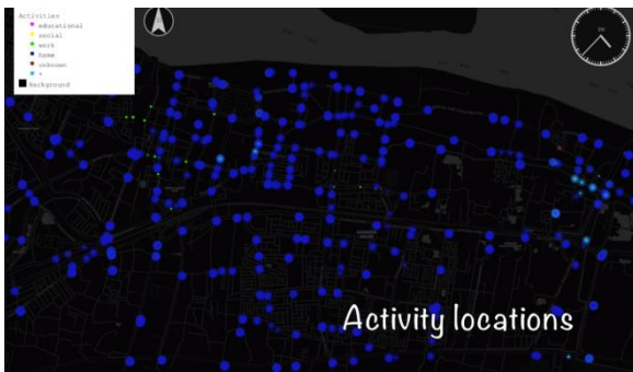
Fig 5- The MATSim also shows the activity location which means the locations of agents at still positions wherever they are working. The agent's locations are indicated by Blue point. MATSim is overall all in one solution which not only simulates but also helps in planning the Big Data Governed urban smart cities.
