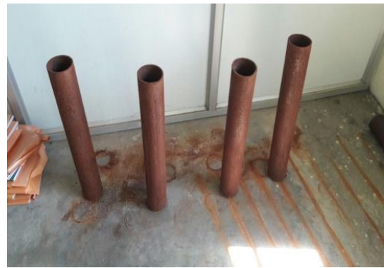
Fig. 2. Some corroded samples.
