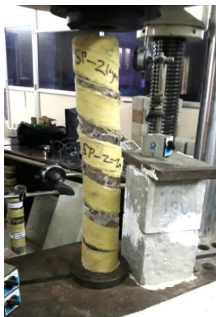
Fig. 7. Failure mode for two layers.
