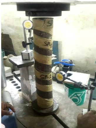
Fig. 6. Failure mode for one layer.
