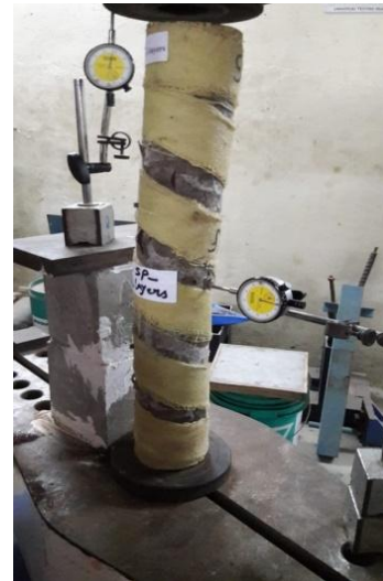
Fig. 8. Failure mode for three layers.
