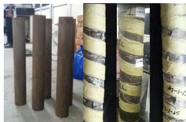
Fig. 3. Samples after surface preparation and AFRP bonding.
