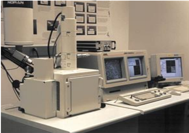
Figure 4: SEM instrument with display monitors showing the microscopic image
