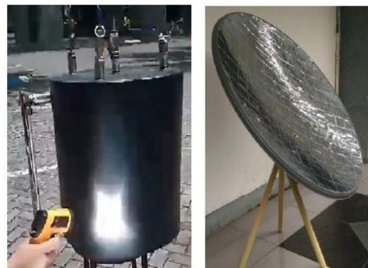
Figure 2. Tools of boiler and solar concentrator
