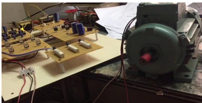
Fig.23: Experimental setup of High step-up converter with a three-phase inverter.
