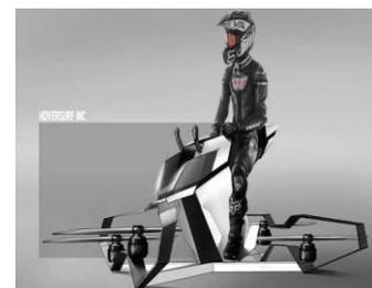
The electric-borne aircraft is intended for both amateur and professional navigators. Hover-surf can carry up to 19 stone in weight while hitting at speeds of 30 miles per hour and reach an altitude of 33 feet.
