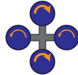
A quad-rotor applies more thrust to one rotor to adjust its pitch or roll and provides less thrust to its diametrically opposite rotors.
