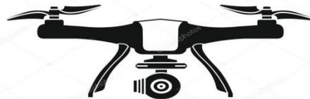
A UAV is defined as a “Powered aerial vehicle” that cannot carry a person, which flies autonomously or by remotely controlled which can carry a lethal or nonlethal payload.
