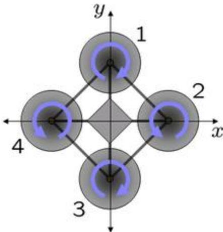
The quad copter hovers or adjusts its altitude as to stable its position while in the air by applying equal thrust to all four rotors.
