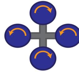
A quad-rotor applies more thrust to one direction rotating rotors as to change its yaw position as to turn its position.
