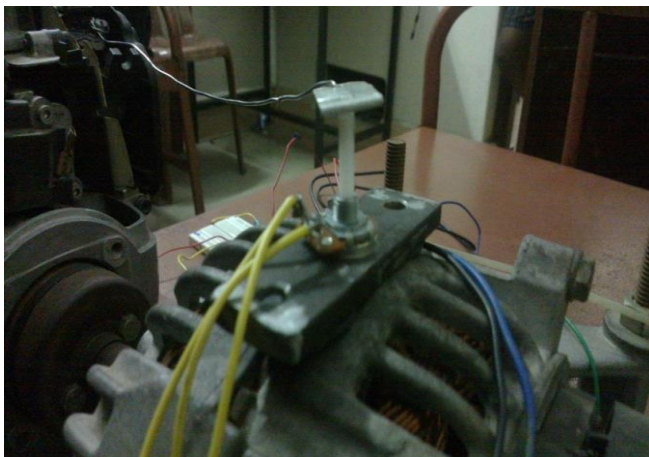
Figure.4 Throttle position sensor in the setup
