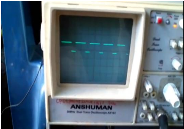
Figure.6. Square waveform of speed obtained in a dual trace oscilloscope
