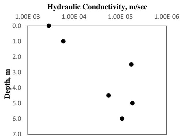
**Figure 7. Hydraulic conductivity variations with depth.**
