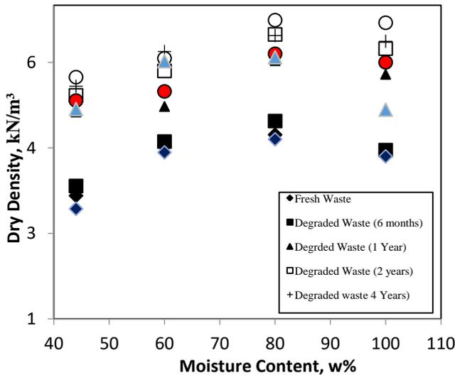
**Figure 5. Comparison of compaction characteristics of MSW (fresh and landfilled waste) from current study with literature.**
