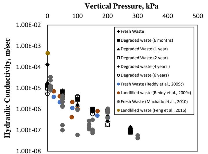
**Figure 6. Variation in hydraulic conductivity of MSW (fresh and old) and comparison with reported literature.**
