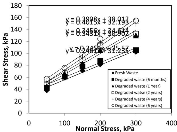
Figure 8. Shear test results for MSW samples (fresh and degraded).
