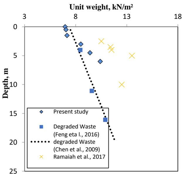
Figure 3. Unit weight variation with depth.
