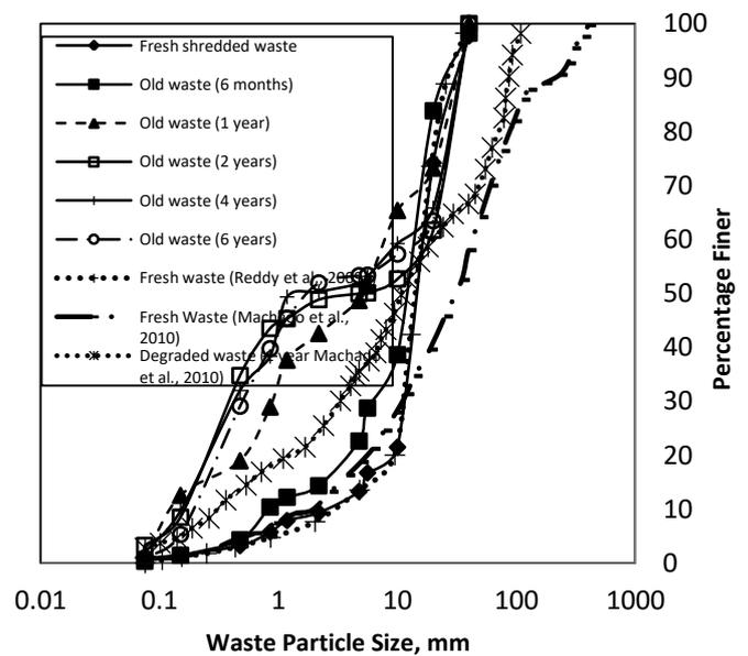
Figure 4. Comparison of particle size distribution of fresh and degraded waste samples of present study with literature.
