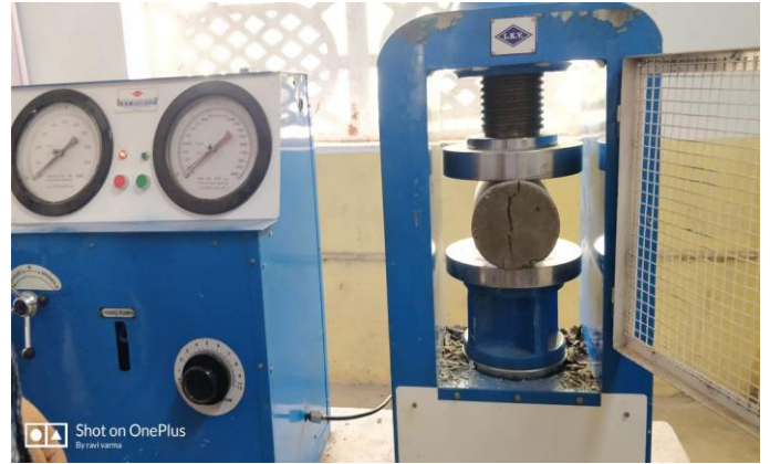
Figure 4: Testing cubes of H_2SO_4 5% Concentration. And 8% Concentration.
