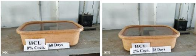
Figure 1: Cubes of HCL 0% Concentration and 2% Concentration.
