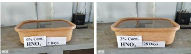
Figure 1: Cubes of HNO_3 0% Concentration and 2% Concentration.
