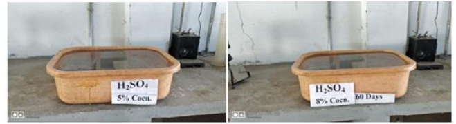
Figure 4: Cubes of H_2SO_4 5% Concentration and 8% Coccentration
