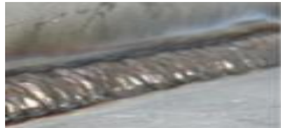
Above figure showing the welded zone of GTAW between SUS304 and AL6061-T6
