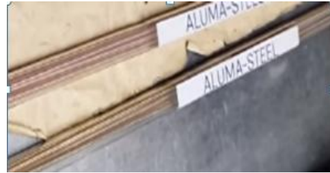
Figure showing welding rod- filler rod
