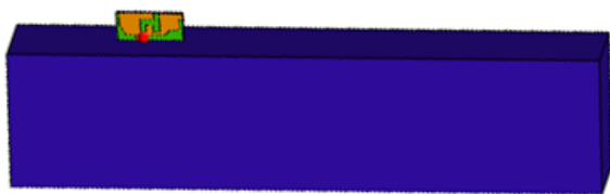
Fig.3 Design of antenna mounted on phantom
