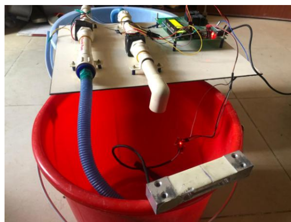
Fig.3 Load Sensor to be placed under the Fuel Tank
