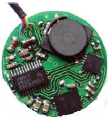
Fig.4. Electronic unit used for on-board processing
