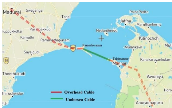
Fig. 3: HVDC transmission line between India & Sri Lanka
