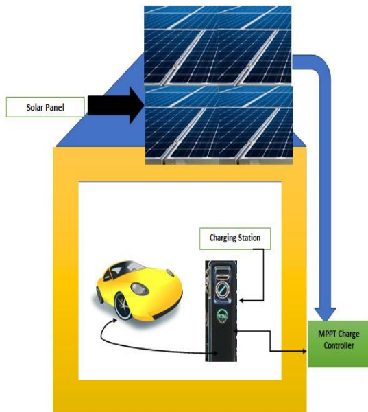
Fig.3: Solar Power Feeding to charging Station
