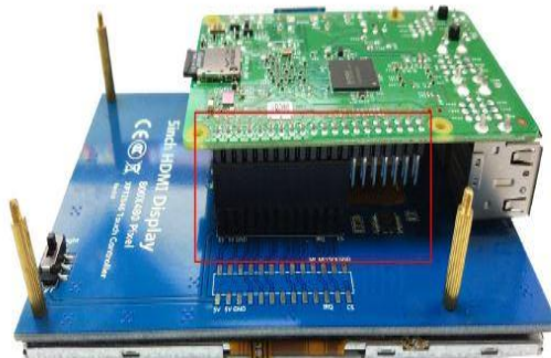
Fig.3: HDMI Display interfaced with Raspberry pi
