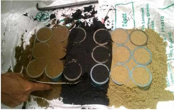
Fig 8. Visual observation of thermally reclaimed, mechanically reclaimed and fresh sand respectively.
