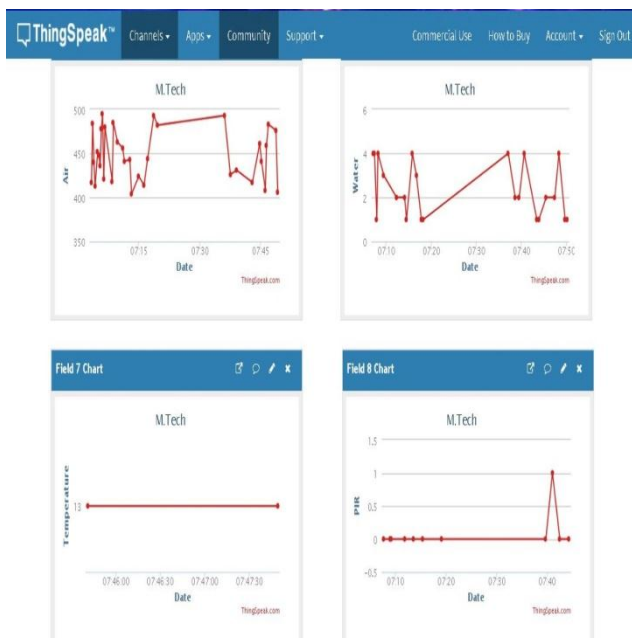
Fig .13.Things speak channels showing gas leakage, water level, temperature and PIR sensor value
