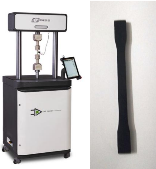
Fig. A.1. Tensile testing setup and test specimen
