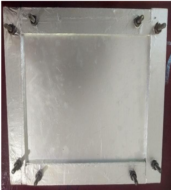
Fig. B.1. Wooden mould wrapped with aluminium foil
