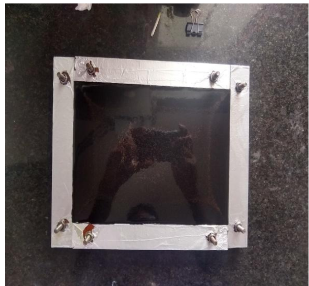
Fig. B.1. Wooden mould wrapped with aluminium foil
