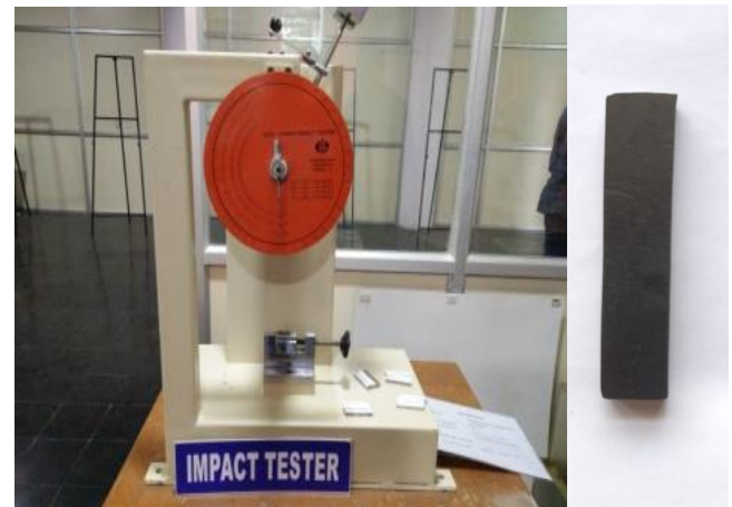
Fig. C.1. Impact test apparatus and test specimen
