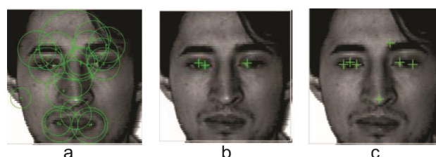
Fig 5 Feature points extracted by using (a) SURF-17points (b) Harris -3points (c) FAST – 7points feature extraction methods
