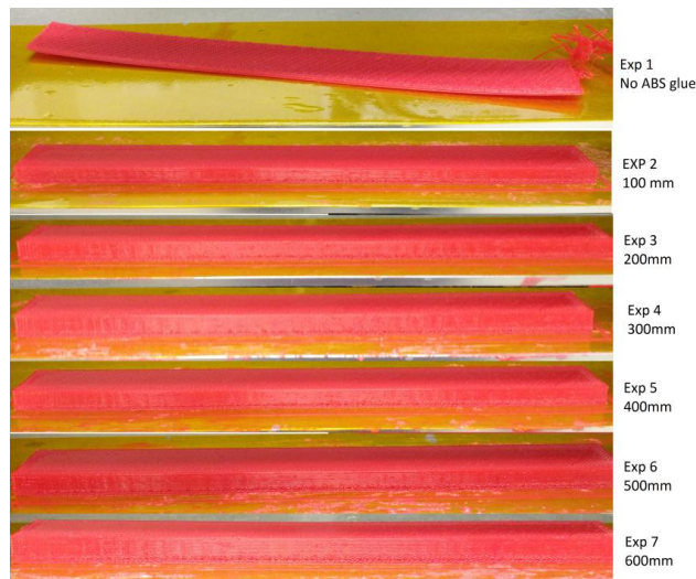
Figure 3: Adhesion between 3D printed rectangular plate with bed
