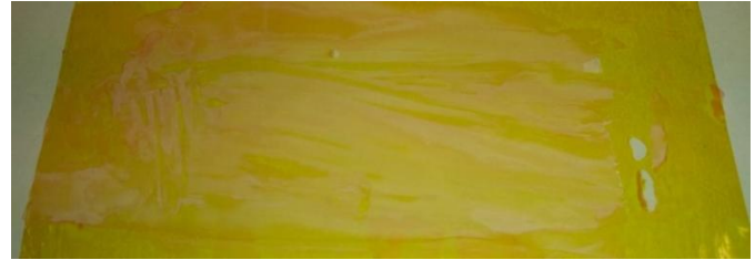
Figure 2: ABS glue applied on a kapton tape
