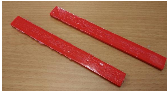
Figure 4: Thin brims at the outline of the printed plates
