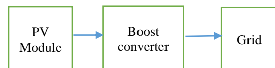
Fig.1. Structure of grid connected PV system.
