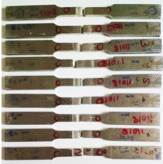
Fig 7: Tensile test Specimens
