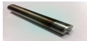
Fig 2: HSS tool used in friction stir welding
