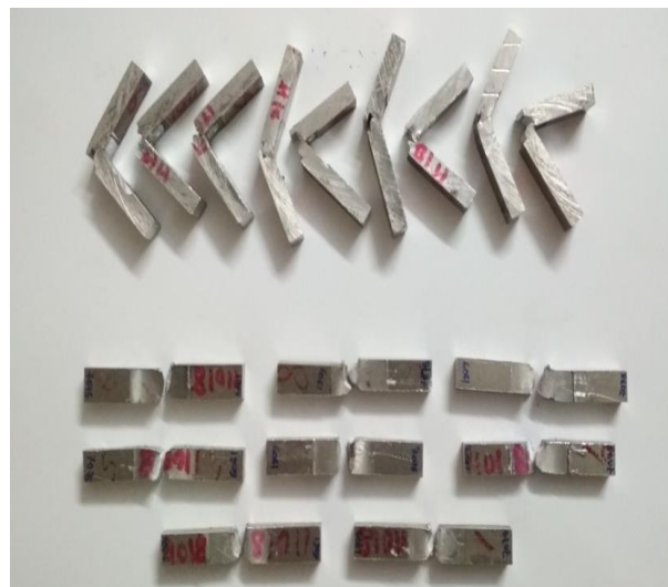
Fig 8: Bending, hardness and impact specimens
