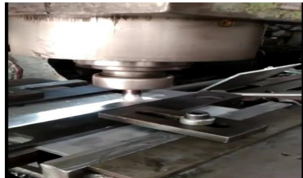
Fig 5: Friction stir Welding of test specimen
