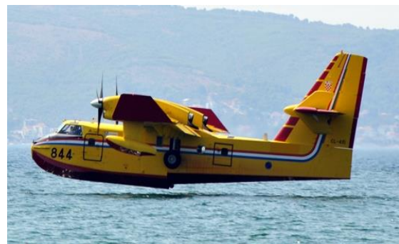
Fig. 1 A seaplane under WIG effect
