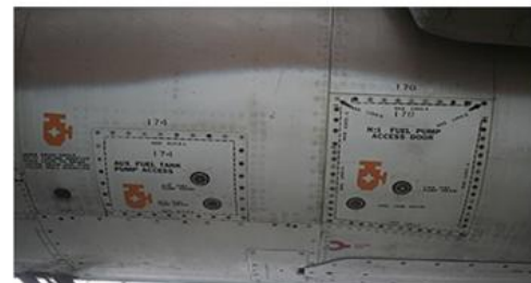
Fig. 1. b) Cut out provided on wings of aircraft.
