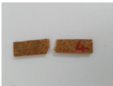
Figure 4 Photographic image of tensile test specimen after fracture.
