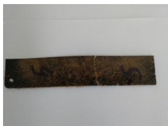
Figure6 Photographic image of flexural test specimen After fracture
