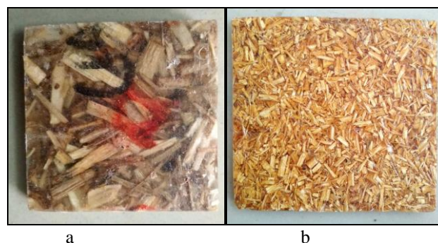
Fig. 3. Photographic view of (a) Morinda citrifolia with Epoxy resin and (b) Morinda citrifolia with Bisphenol resin.
