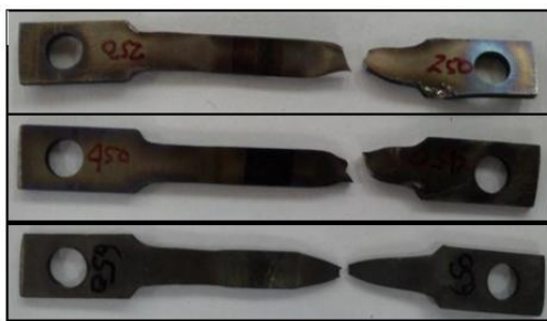
Figure 8: tensile fractured specimens
