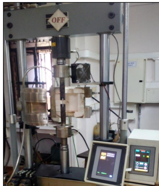
Figure 5(b): tensile test at elevated temperature of 250°C, 450°C and 650°C
