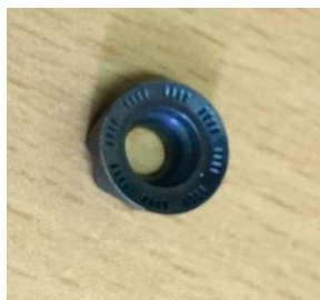
Fig II. Tungsten Carbide Cutting insert
