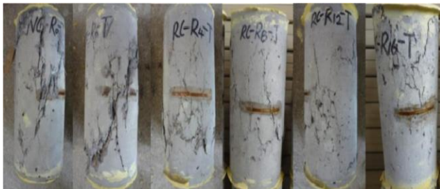
NC-RO RC-RO RC-R4 RC-R8 RC-R12 RC-R16 (a) Failure mode of mixes exposed to 25°C
