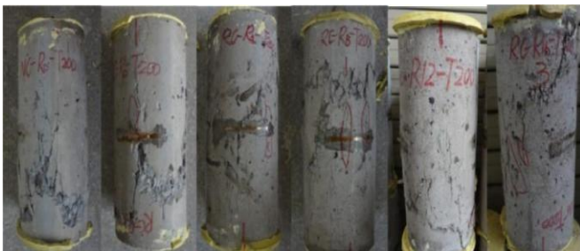
NC-RO RC-RO RC-R4 RC-R8 RC-R12 RC-R16 Failure mode of mixes exposed to 200°C
