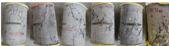
Failure mode of mixes exposed to 400°C
