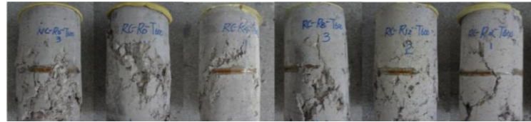
NC-RO RC-RO RC-R4 RC-R8 RC-R12 RC-R16 Failure mode of mixes exposed to 600°C
