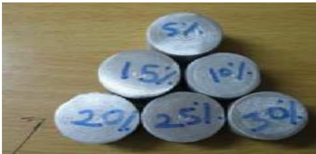
Figure 3. Specimens for hardness test of Metal Matrix Composite
