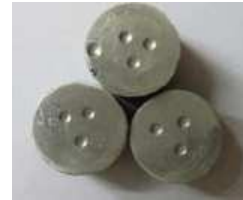
Figure 5. Specimens of hardness tested of Metal Matrix Composite
