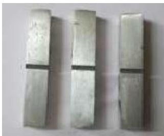
Figure 4. Specimens for Impact test of Metal Matrix Composite
