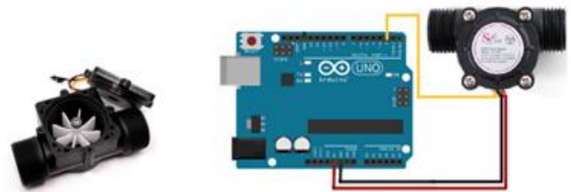
Fig. 4 Water flow sensor, arduino and circuit diagram [8]
