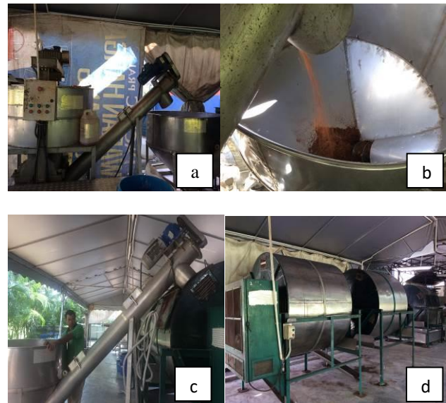
Fig. 1: The (a) Mixer and Shredded machine; (b) shredded food waste, (c) feeding shredded food waste into Rotary Compost Drum and (d) Rotary Compost Drum.
