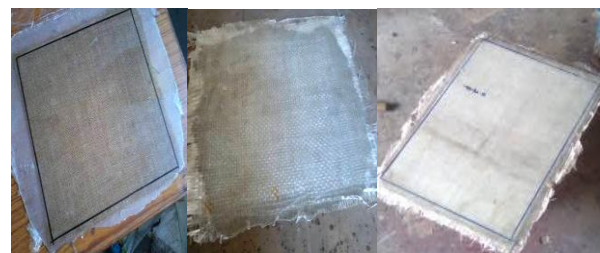
Fig.2 Laminates after curing 24 hours
