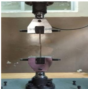
Fig. 3 Specimen held between the gripper jaws of UTM
