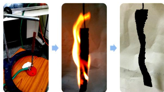
Figure 7 Flame resistance test of the composites
