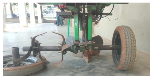
Fig 2: Univaersal shaft with rotavator and wheel assembly
