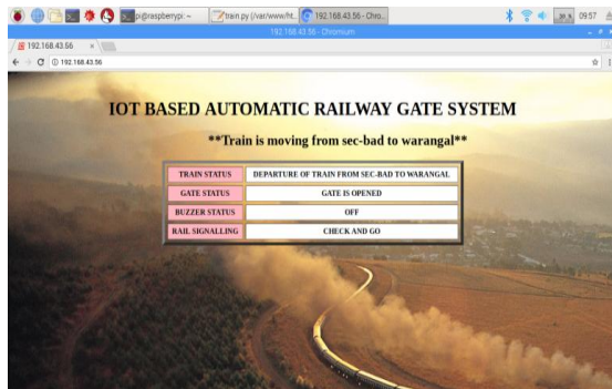
Fig 8: IoT based Application monitoring for railway level crossing
