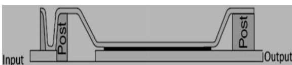
Fig. 3: Shunt capacitive switch in Down-state.
