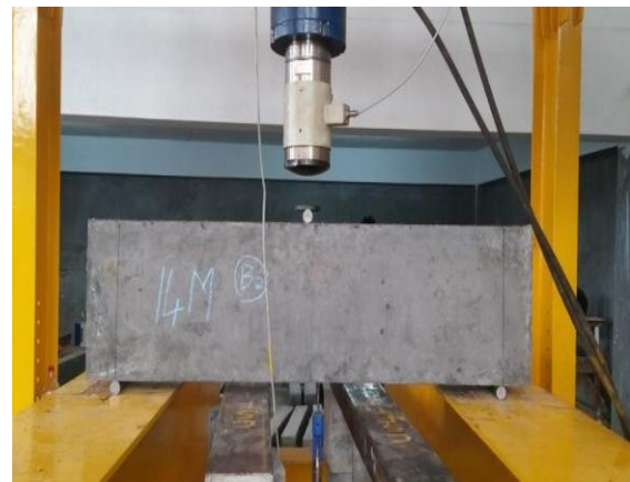
Fig.1: Three point bending test setup.
