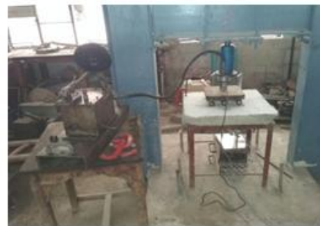
Fig 3&4: Experimental set up for flexural behavior of slab
