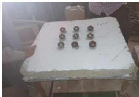
Fig 3&4: Experimental set up for flexural behavior of slab
