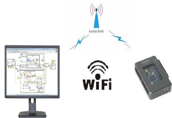
Fig. 3. Connection of myRIO-1900 with host system
