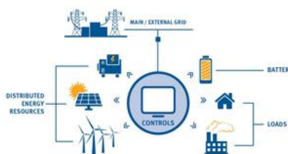
Fig. 1. Central Controller for Microgrid
