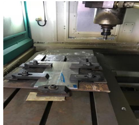
Fig. 6: FSW Welding Experiment Setup on VMC
