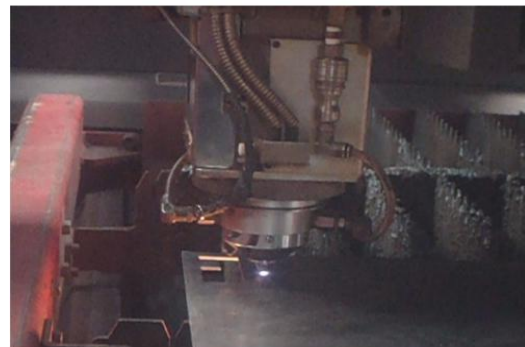
Figure .1. The CO 2 laser cutting machine And also significant parameters are considered for Laser beam power, gas pressure and cutting speed.
