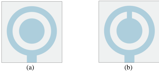
Fig. 1. O-shaped antenna in different configurations: a) Step 1 (OFF state), b) Step 2 (ON state)
