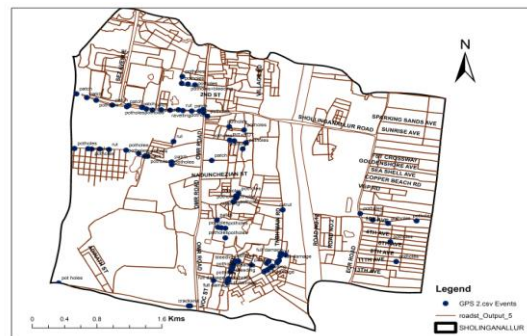
Figure 6 Points Locating Distresses
