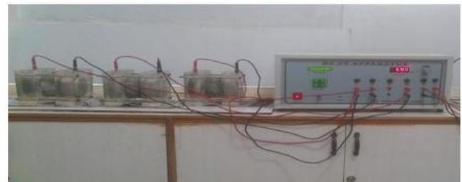
Fig .5 RCPT test of cube specimen
