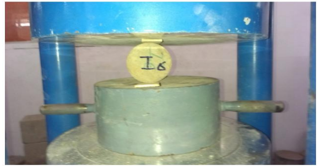
Fig.3 Split tensile strength test of cylinder
