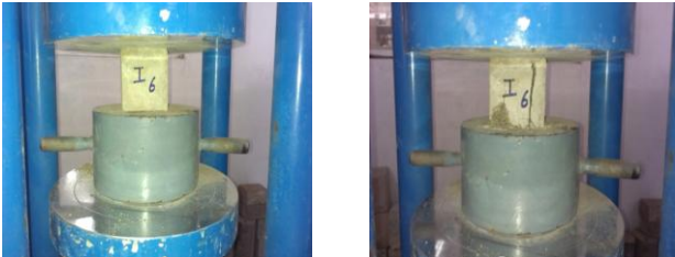
Fig.1 Compression strength test of cube
