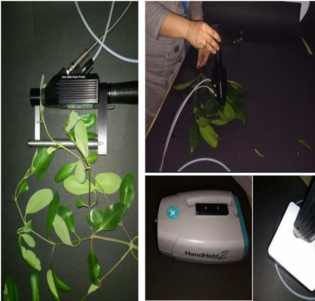
Fig.5.2 Spectra collection using HandHeld 2 Spectroradiometer
