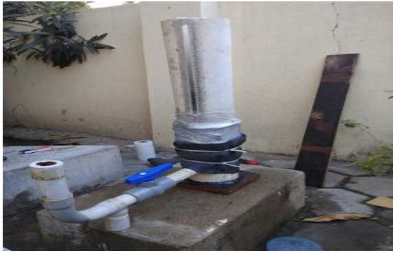
Fig.1- Test setup for falling head Method
