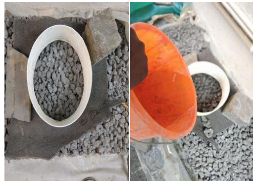
Fig.3- Test setup for Infiltration rate of sample (a) placement of ring, (b) Water is poured in the ring
