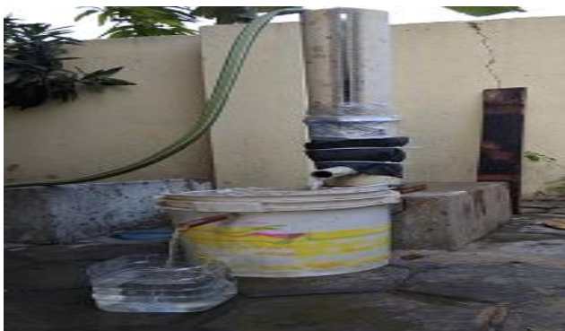
Fig.2- Test setup for Constant head Method
